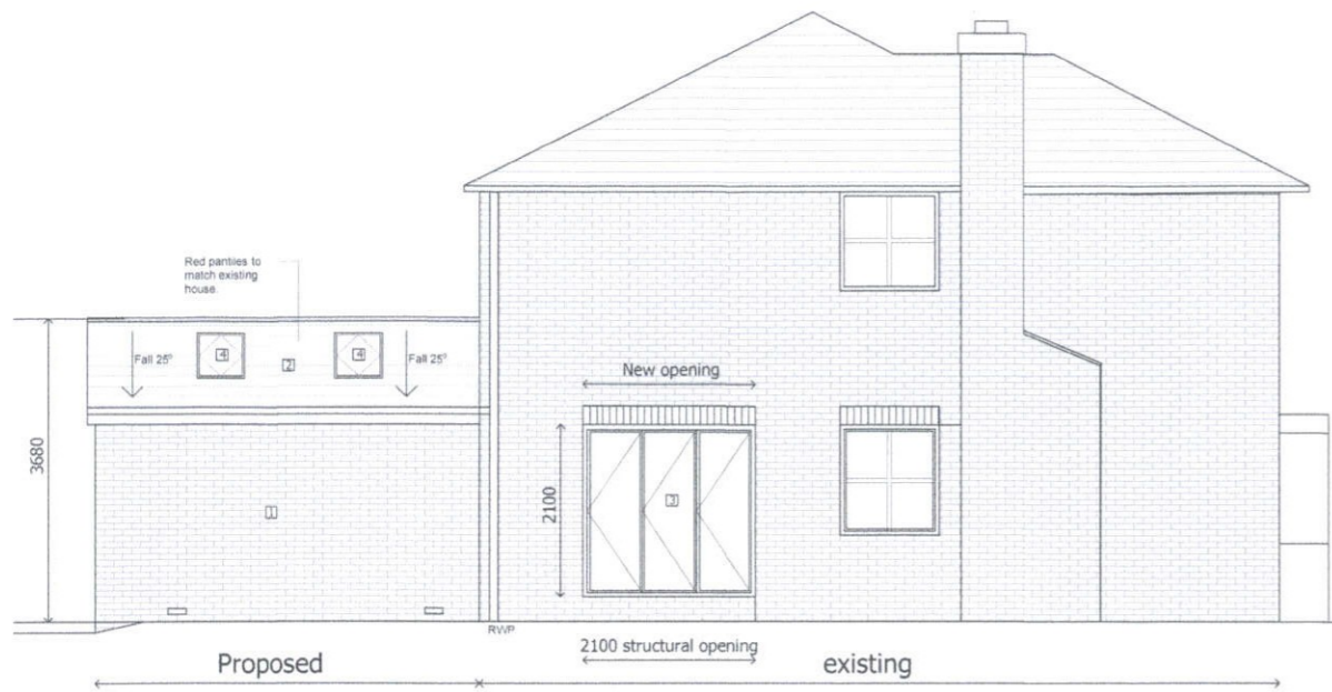
Proposed Side Elevation AA 1:50
