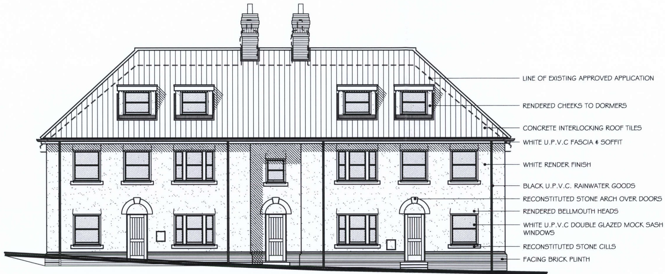
NORTH-WEST ELEVATION (TO HOCKLEY ROAD) 1:100
