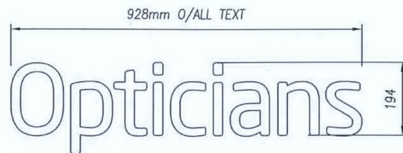
DETAIL ELEVATION (SCALE 1:10)
