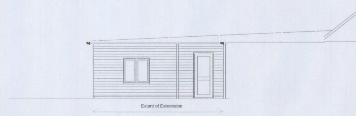
COURTYARD SECTIONAL ELEVATION TOWARDS NEW OFFICE
