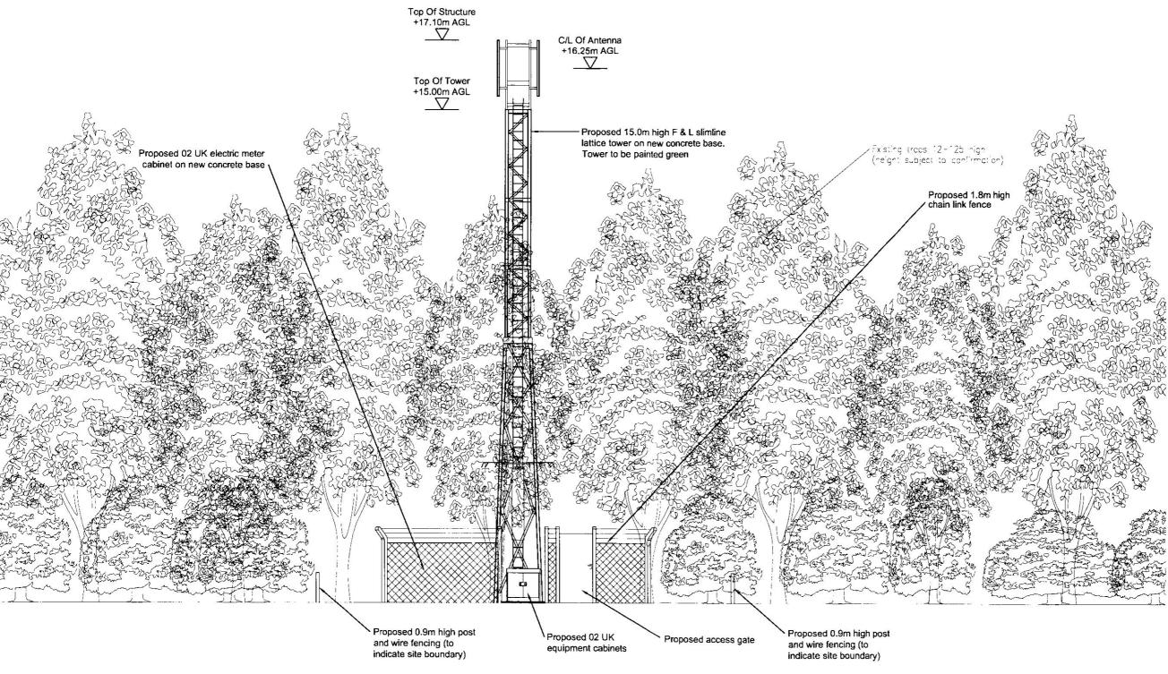
East Elevation Scale 1:100 Use figured dimensions only, do not scale from drawing.
